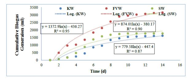
Figure 6. Comparative Results for KW, FVW and GW Biogas Production
