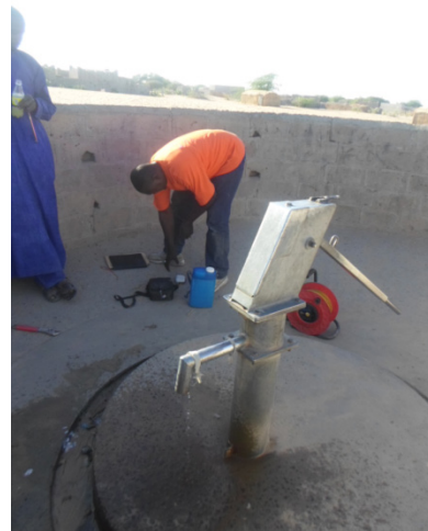
Figure 3. Boreholes used for water level measurements
