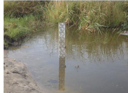
Figure 5. One of the limnometric scales installed in Bol (northeast of Lake Chad)
