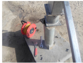
b) Move the upper part, drilling Leaving space to introduce the probe.
