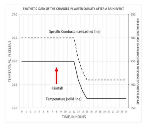
Figure 5. Synthetic data and shows what will happen to the pumped water if the old aquifer water has a temperature of 26  $^{\circ}$ C and a specific conductance 500  $\mu$ S/cm
