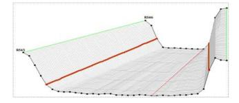
Figure 3.b.Interpolated cross-sections plots Between RS46 and RS45
