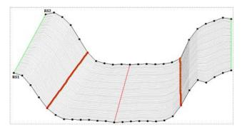
Figure 3.c.Interpolated cross-sections plots Between RS2 and RS1
