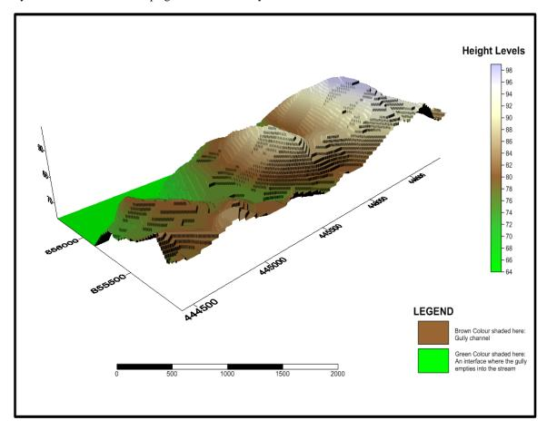
Figure 2: Digital elevation model showing morphology of the studied gully system
