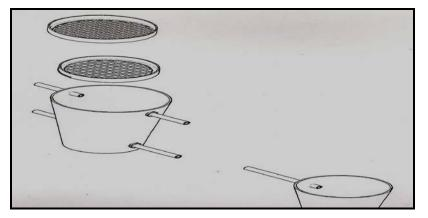
Figure 7. Assembly drawing showing the arrangement of filter elements of the plant
