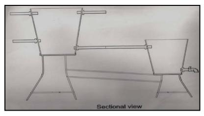
Figure 6. Sectional view of the filtration plant
