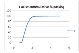
sharp sand used for water filtration. Sand grains retained by sieve size 1.18mm-0.710micron was used to enable sand properly trap minute contaminants and still allow sufficient water flow rate.
