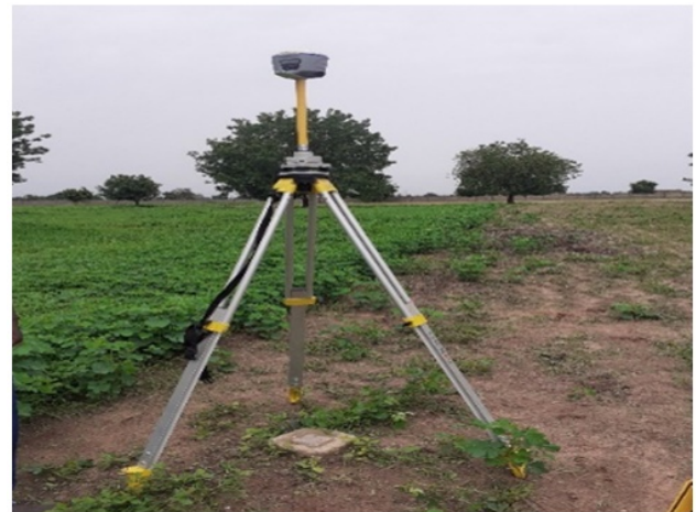
Figure 6. i50 GNSS receiver stationed as a base at point B118
